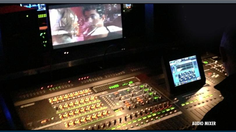
Audio includes: a Yamaha PM-5DRH with Genelec speakers and a Riedel Artist-64 digital intercom system. Tape rack #1 can support up to 10 VTRs and includes a Playback-Pro file based video playback system (additional playback options are: EVS, 3-Play and/or Fast-Forward).
